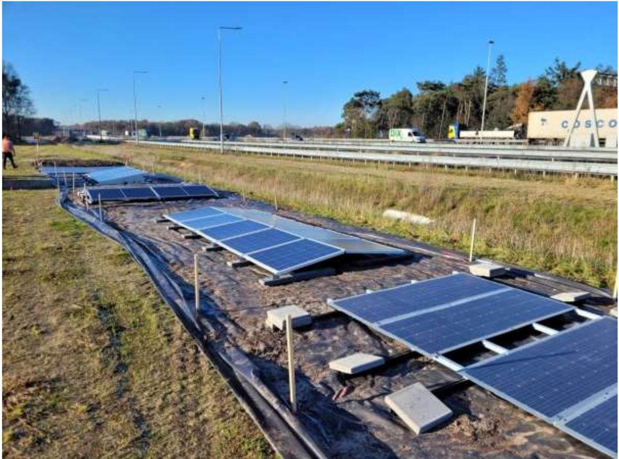
**Rijkswaterstaat is investigating the possibility of laying solar panels horizontally in road berms without the need for installing a crash barrier. We refer to this as ‘obstacle-free solar panels’.**
